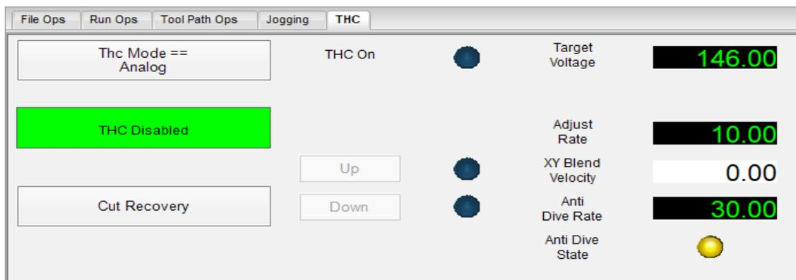
This tab contains run time info as well as DROs that will be used to set optimal cutting conditions.
