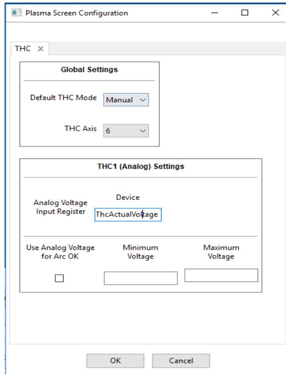
In our example, the motion controller outputs an analog signal. Analog should be selected as default. Manual mode will still be available. The analog voltage is a register that can be found by going to Diagnostics>Regfile and selecting your motion controller, then its plasma unit. If the Register is clicked on with the diagnostics open, Mach4 will display the full path name. When Mach4 is restarted
